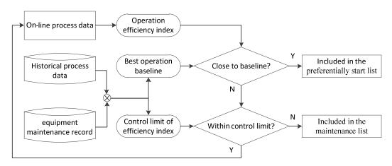
Fig.2. Flow chart of compressor and inter cooler monitoring.
