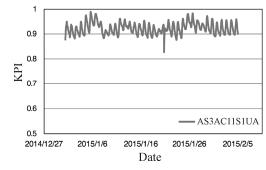
Fig.6. Efficiency of AS3AC11S1 intercooler.
