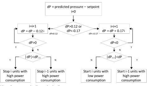
Fig.1. Algorithm of compressor loading and unloading.
