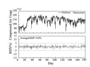
Fig.4. Prediction result of PA consumption after correction.
