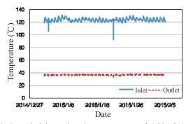
**Fig.7.** Air inlet and outlet temperature of AS3AC11S1 intercooler.
